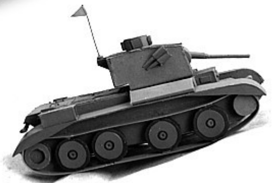
Option: mantlet spaced armour on Mk IV turret
